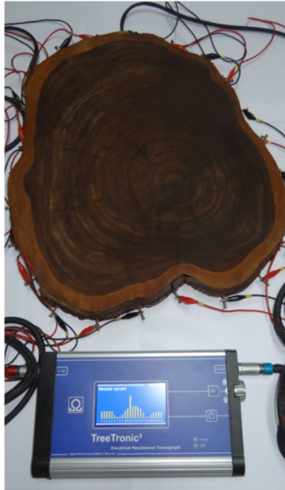
Figure 1. The Electric Resistance Tomograph (ERT) is connected to a moist teak disc.
