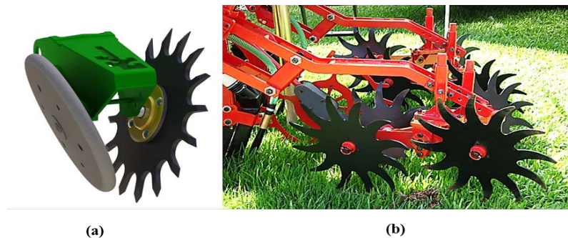
Figure 6. Finger wheels associated with compactor wheels (a) and in pairs (b) Photos: (a) Martin Industries Catalog, (b) A. Araújo.
