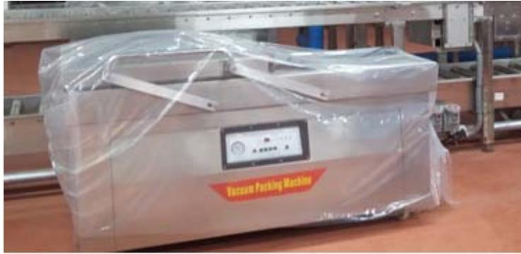
Figure 7. Automatic vacuum packaging machine.
