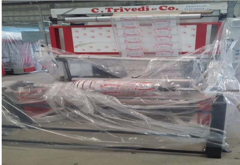
**Figure 4. Printing machine for printing necessary information on plastic materials.**
