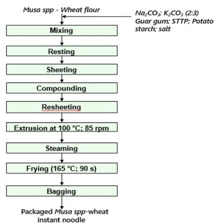
**Figure 2. A schematic diagram showing production of fried instant noodle.**
