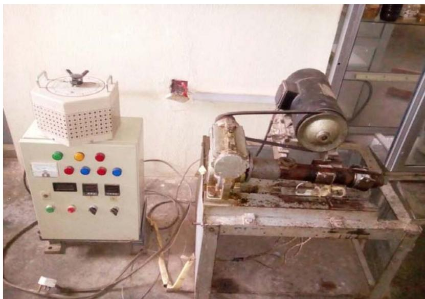
Plate 3. A laboratory model rotating screw extruder.
