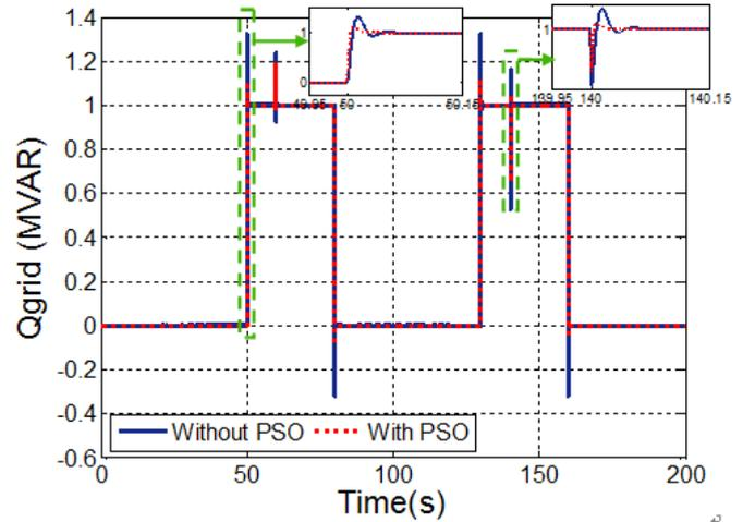
Fig. 11. Reactive power injected to grid.
