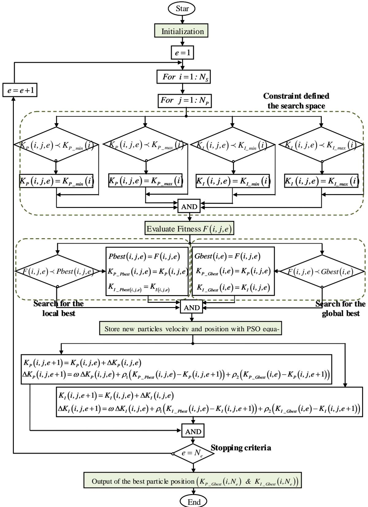
**Fig. 3.** Detailed diagram of the OMFPSO algorithm.
