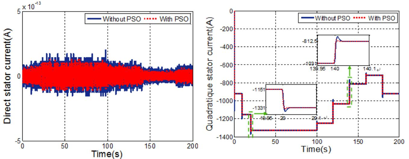
Fig. 7. The d-q components of the stator current.
