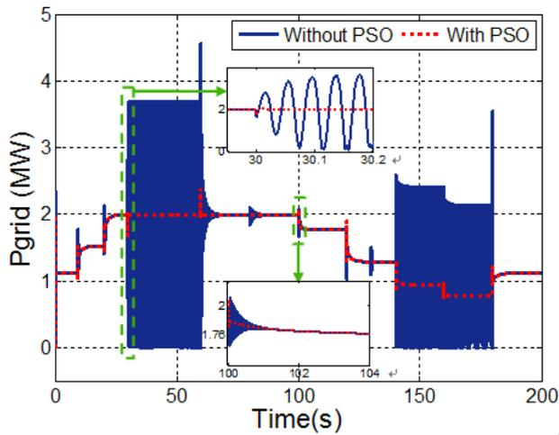
Fig. 10. Active power injected to grid.
