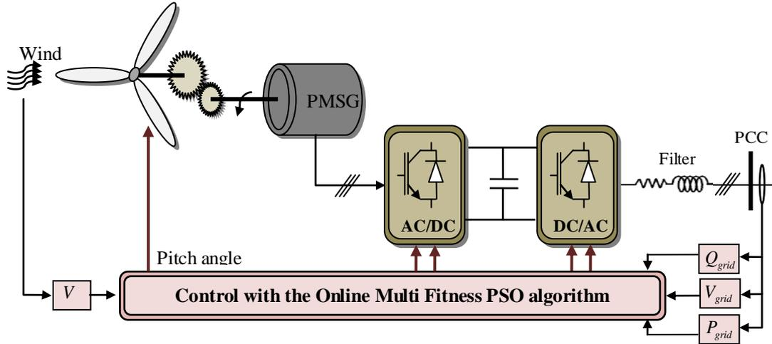
Fig. 1. Schematic diagram of the WT conversion system.
