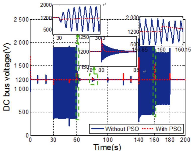
Fig. 8. The DC bus voltage.
