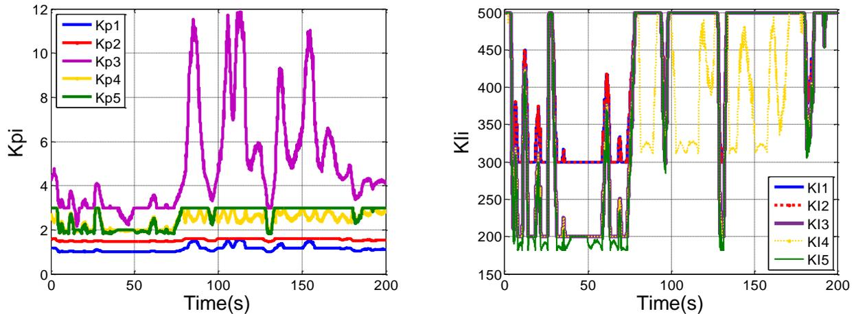
**Fig. 5.** PI parameters variation under variable wind speed.
