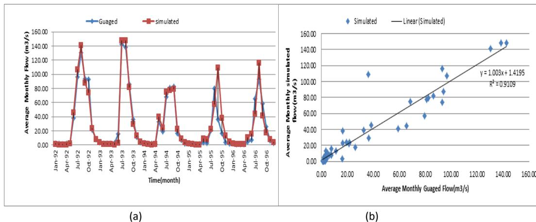
**Figure 10: Calibration result of average monthly simulated and gauged flows (a) and Scatter plot of monthly simulated versus gauged flow (b) at the outlet of the watershed**
