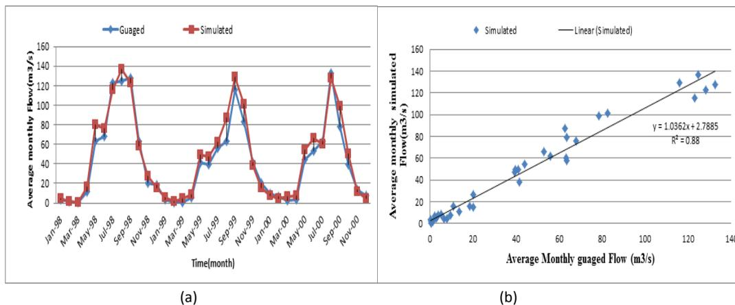
**Figure 11: Validation result of average monthly simulated and gauged flows (a) and Scatter plot of monthly simulated versus gauged flow (b) at the outlet of the watershed**
